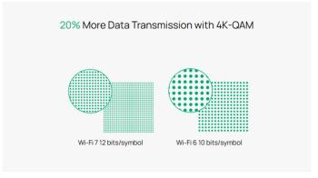
4096-QAM enables each symbol to carry 12 bits instead of 10, increasing theoretical transmission rates by 20% compared to Wi-Fi 6's 1024-QAM. This higher transmission rate boosts data throughput, delivering enhanced speeds and improved network reliability.
